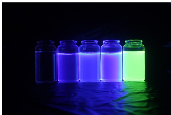
Figure 13. Light is emitted from five samples illuminated by UV lamps. From left to right, pure water ( H_2O ), PPO, POPOP, bis-MSB, and 6-FAM samples. Pure water did not emit any light. A cylindrical quartz container was filled with WbLS using Triton X100 surfactant.
